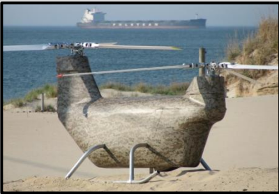
Self-launch/land in unprepared terrain; Intake filters protect engine from FOD
